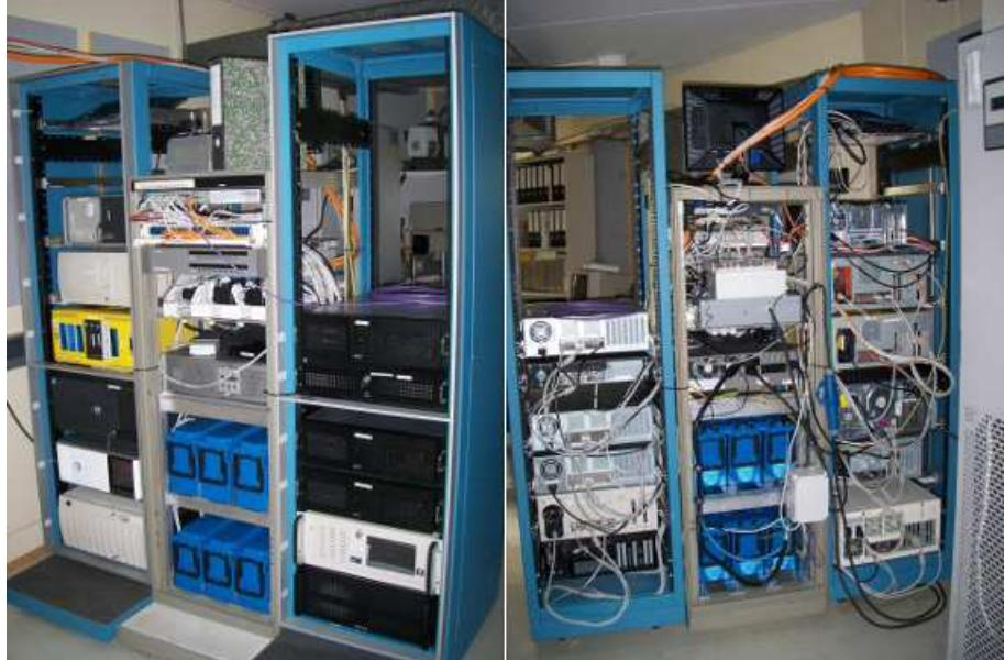
Figure 2: Front and back views of the new server rack. On top of the middle rack: webcam pointed at the extra display (keyboard and main display are on a table on the front side of the rack). In the middle rack, from top to bottom: gigabit ethernet switch, media converters for internet and clock cellar fibers, fiber optic panel, KVM switch, controllable power sockets, remote keyboard device and its controller computer, UPS, UPS extra batteries.
