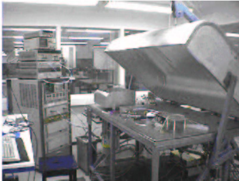
Figure 2: EM-receiver test system with open cryochamber.
