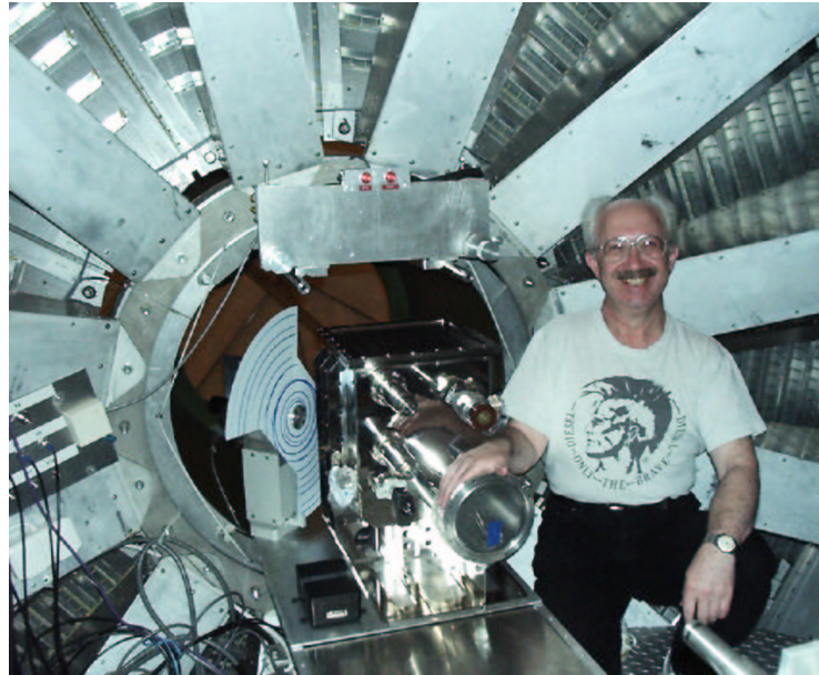
Figure 3: Picture of the 3/2 mm SIS receiver on the antenna.
