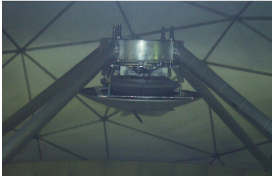
Figure 5: Picture of the subreflector with the supporting structure.
