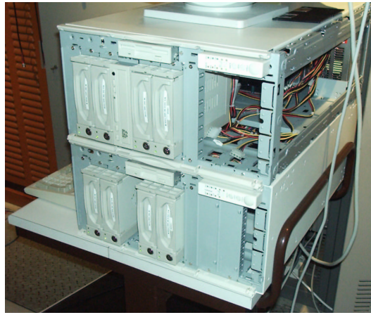
Figure 9: The two-PC prototype used to record gigabit VLBI data.
