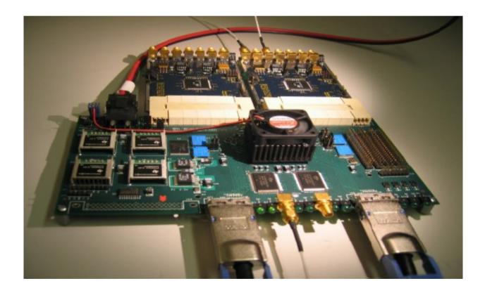
Based on the inexpensive iBob board by UC Berkeley. Gigabit A/D samplers allow very wide bandwidth => much improved VLBI sensitivity! The 2x10 Gbps LAN makes it e-VLBI -ready.
