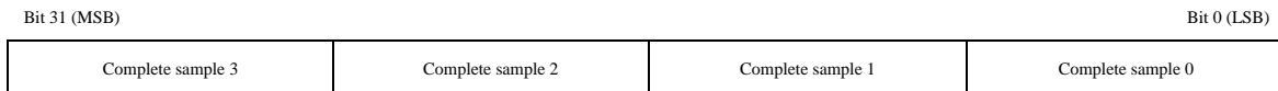
Figure 17: Data Array word for complete-sample length of 8 bits (i.e. 2^n * 2^k = 8 ); relative sample times are indicated in each 8-bit complete sample
